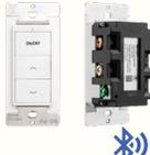
KEILTON WP1013S LINE VOLTAGE 3 BUTTON BLUETOOTH DIMMER SWITCH                      | Switch on/off or dim an individual light or a group of lights (defined in the commissioning App) 120-277v AC powered.                                 | Field installed, ideal for retrofitting existing wall switch, neutral wire is required, indoor. <b>not to serve as circuit switch.</b> |
