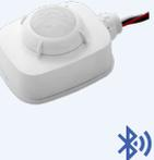
KEILTON EFS104 LINE VOLTAGE BLUETOOTH MESH NODE W/ PIR DLH SENSOR           | Enable network controlled - on & off, dim, trim, zone, group, scene & schedule, etc. And, PIR occupancy & daylight (harvesting) sensing  | works with PacLights dimmable fixture(s), total up to 1200w (120-277v), indoor/outdoor           | Field installed, Fixture mount                       |
