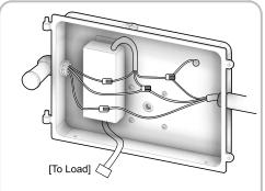
5. Make all connections inside the back box of the FWPT and must be compliant to NEC standard. All connections must be made by a qualified electrician.
