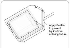
6. Once all wiring is complete. Fasten the Cover to the Junction Box. Add Sealant on all connections. (Not Included)
