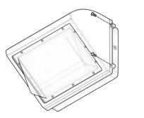
Remove the (2) screws on the right side of the fixture to remove the back box from the pins on the front housing. Disconnect the wiring from the front of the fixture and the LED Driver.
