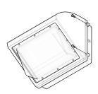
1. Remove the (2) screws on the right side of the fixture to remove the back box from the pins on the front housing. Disconnect the wiring from the front of the fixture and the LED Driver.
