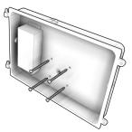
3. Fasten the FWPT Back panel to the mounting surface using mounting screws. (not included). Make sure to align the conduit opening to the hole in the wall.
