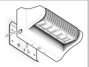
4. Once the back plate is properly secured. Clip the FWPR fixture to the back plate by inserting the two tabs on the plate to the two slots.
