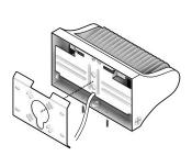
1. Remove the (2) screws on the bottom side of the fixture to remove the backplate from the fixture.
