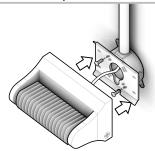
4. Once all wiring is properly installed, Fasten the back plate with felt pad to the junction box cap. (Fasteners not included)
