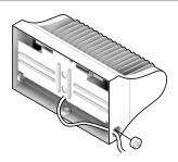
2. Determine where the power supply cable conduit will be installed to the FWPR fixture. Run the cable through of the the three holes and remove cap.
