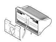
1. Remove the (2) screws on the bottom side of the fixture to remove the backplate from the fixture.
