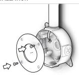
2. Install a plastic junction box cover with [4] mounting holes and one center hole to run cables. Fasten [2] screws to the junction box.
