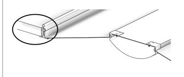
**STEP 3b:** After the frame is properly installed to the ceiling, one can then mount the FTFB luminaire. It is recommended to also attach a safety aircraft cable to provide an extra degree of safety. Please refer to wiring diagram for wire installations.
