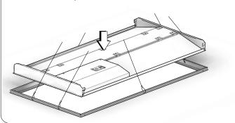
STEP\_2b: If the drywall ceiling is at least 1" Thick, then the Drywall Kit can be fastened from the holes provided. All mounting screws are not included.
