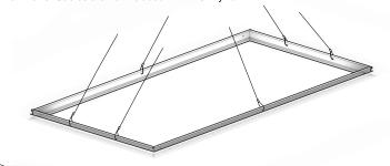
STEP 3: Carefully mount the FTFB to the recessed frame and adjust any aircraft cables if its neccessary.
