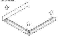
STEP 3: Slide in the FTFB luminaire through the open side of the Surface Mount Kit. This is when all the wiring installations should be made as well. Please see the wiring diagram on the front page for wire installation instructions.
