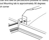
2. Use side cutters to adjust each tab to height of T-grid.
