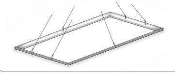
**<u>STEP</u> 2b:** If the drywall ceiling is at least 1" Thick, then the Drywall Kit can be fastened from the holes provided. All mounting screws are not included.
