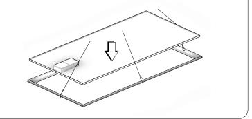
**STEP 3b:** After the frame is properly installed to the ceiling, one can then mount the FPAN luminaire. It is recommended to also attach a safety aircraft cable to provide an extra degree of safety. Please refer to wiring diagram for wire installations.
