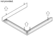
STEP 3: Slide in the FPAN luminaire through the open side of the Surface Mount Kit. This is when all the wiring installations should be made as well. Please see the wiring diagram on the front page for wire installation instructions.
