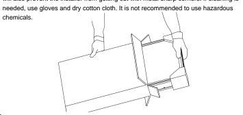
2. Lift up four ( four for 2x2, six for 1x4 and 2x4) mounting clips on the sides of the luminaire. You can do it by hand (Do wear work gloves) or use pliers.
