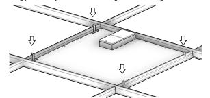
Remove electrical enclosure cover Carefully remove knockout for AC line input wires and 0-10 V control line. Install listed electrical fitting in the knockout holes for wire protection if needed.
