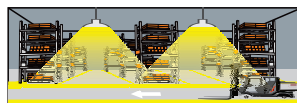
With insufficient ambient light, the sensor will turn on the lighting fixture when motion is detected.
