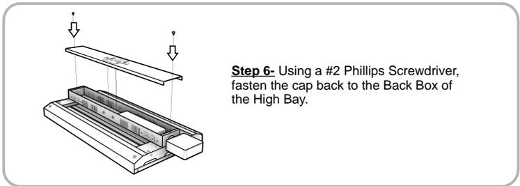
**Step 6-** Using a #2 Phillips Screwdriver, fasten the cap back to the Back Box of the High Bay.
