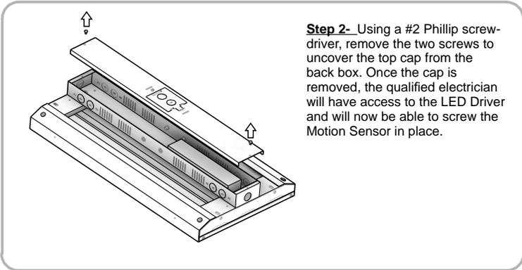
**Step 2-** Using a #2 Phillip screwdriver, remove the two screws to uncover the top cap from the back box. Once the cap is removed, the qualified electrician will have access to the LED Driver and will now be able to screw the Motion Sensor in place.
