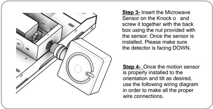
**Step 3-** Insert the Microwave Sensor on the Knock out and screw it together with the back box using the nut provided with the sensor. Once the sensor is installed. Please make sure the detector is facing DOWN.
