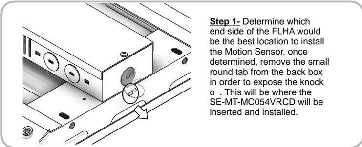
**Step 1-** Determine which end side of the FLHA would be the best location to install the Motion Sensor, once determined, remove the small round tab from the back box in order to expose the knock out. This will be where the SE-MT-MC054VRCD will be inserted and installed.
