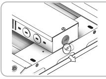
Step 1- Determine which end side of the FLHA would be the best location to install the Motion Sensor, once determined, remove the small round tab from the back box in order to expose the knock o. This will be where the SE-MT-MC054VRCD will be inserted and installed.
