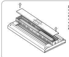
Step 2- Using a #2 Phillip screwdriver, remove the two screws to uncover the top cap from the back box. Once the cap is removed, the qualified electrician will have access to the LED Driver and will now be able to screw the Motion Sensor in place.
