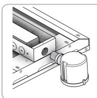
Step 3- Insert the Microwave Sensor on the Knock o and screw it together with the back box using the nut provided with the sensor. Once the sensor is installed. Please make sure the detector is facing DOWN.
