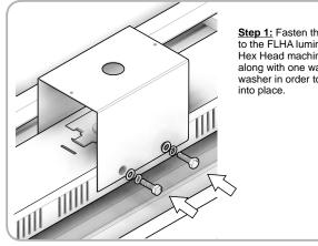
Step 1: Fasten the FLHA-ME bracket to the FLHA luminaire using the Hex Head machine screws provided along with one washer and lock washer in order to screw the bracket into place
