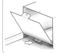
Step 3: Once all wiring is complete, use the two cover tabs that are provided to cover the sides of the Pendanct bracket. Step 4: Use the two remaining screws to fasten the cover plates into place.
