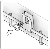
Step 2- Use the four [4] formed tabs to fasten the wire guard onto the light fixture. This is done by using the 4 holes located on the side parts of the luminaire.
