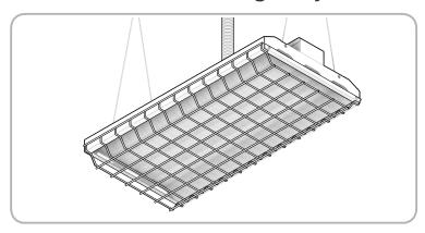
Step 1- The FLHA luminaires are made in various sizes. It is important to make sure that the wire guard is the corresponding size based on the luminaire chosen.
