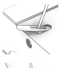
Step 3- Using the shorter aircraft cable (with two tabs on both ends), insert the two slot-shaped tabs into the FLHA slots on both sides. This is accomplished by first inserting one end of the tab and using the slot to move the cable as desired to bring in the second end of the tab. Once this tab has been inserted into the luminaire, it will be safely secured into place for mounting.
