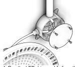
4. Run the LED driver cable from the FHUP into a junction box with 100-277 VAC power supply cable and complete the wiring.
