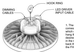
1. The FHUP luminaire comes with a ring hook which can be used to hang the fixture to a desired height. Screw in the ring hook into the back threaded hole in
