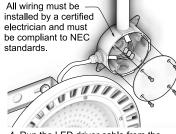
4. Run the LED driver cable from the FHUE into a junction box with 100-277 VAC power supply cable and complete the wiring.
