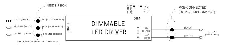
3. All wiring connections must be made inside a Junction Box. Make sure to choose the correct junction box for the desired application. Some junction boxes are made for outdoor applications and others are made for indoor applications.
