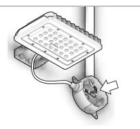
5. Follow the Wiring Diagram and properly wire the FFLA fixture to the power supply cables. Make sure the fixture is connected with the appropriate voltage power supply. All wiring must be installed by a certified electrician and must be compliant to NEC standards.
