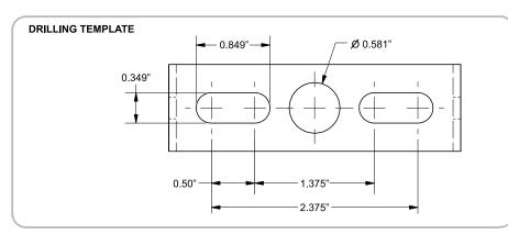
1. Drill holes on the mounting surface by following the Drilling Template to mount the AC-FLA-TM Trunnion mount to the desired height. (Keep the mounting location close the where the junction box is located.)
