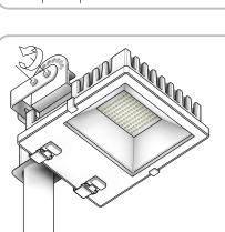
2) After properly securing the FFL to the pole with the Slipfitter, Use a wrench to remove the bolt located on the arc of holes on the side of the FFL. Once the Bolts have been removed from both sides of the FFL, the fixture will be able to rotate. Adjust the tilt on the luminaire to the desired angle. Refasten the bolts to a location that will lock the position desired.
