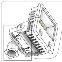
1) Loosen the [2] M8-1.25 Hex Head Bolts from the ACFLSF Slipfitter Mount. Align the Slipfitter to the FFL Handle and fasten the two pieces together using the [2] Hex Head Bolts and washers.
