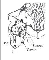
G After properly securing the FFHS/2 Luminaire with the Slip Fitter to the pole, if needed, adjust directly at the Slip Fitter by removing the Phillips head screws, the cover, loosening the bolt with a wrench, and pulling slightly to move the parts freely from the teeth. After adjusting the Slip Fitter tilt, mate the parts at the teeth and fasten the bolt, put the cover in place, install the screws.
