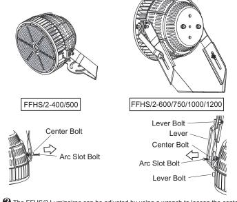
② The FFHS/2 Luminaires can be adjusted by using a wrench to loosen the center bolts and the arc slot bolts located on the sides of the FFHS/2 Luminaire. The FFHS/2-600/750/1000/1200 Luminaires will also need the lever bolts located on the sides of the FFHS/2 Luminaire to be loosened. The fixture will now be able to rotate to the desired tilt/angle. Replace the arc slot bolts and tighten all the other bolts.
