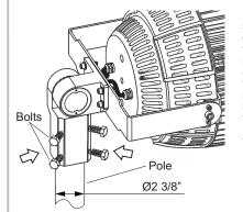
Once the Slip Fitter is properly secured onto the FFHS/2 Fixture, one can then run the Power Cable from the Fixture to the inside of the pole to allow it to be powered with an AC Power Supply Cable. Follow the wiring diagram. One can then place the Slip Fitter on top of a standard 2 3/8" diameter pole, adjust the orientation and fasten the [4] Hex Head Bolts to secure the Slip Fitter to the pole.
