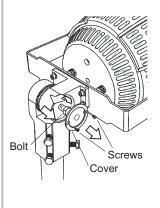
After properly securing the FFHS Luminaire with the Slip Fitter to the pole, if needed, adjust directly at the Slip Fitter by removing the Phillips head screws, the cover, loosening the bolt with a wrench, and pulling slightly to move the parts freely from the teeth. After adjusting the Slip Fitter tilt, mate the parts at the teeth and fasten the bolt, put the cover in place, install the screws
