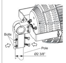
Once the Slip Fitter is properly secured onto the FFHS Fixture, one can then run the Power Cable from the Fixture to the inside of the pole to allow it to be powered with an AC Power Supply Cable. Follow the wiring diagram. One can then place the Slip Fitter on top of a standard 2 3/8" diameter pole, adjust the orientation and fasten the [4] Hex Head Bolts to secure the Slip Fitter to the pole.
