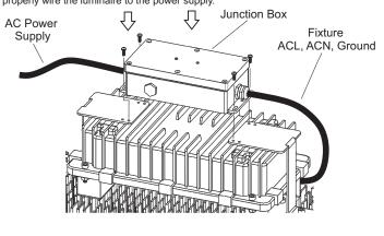
Using a J-Box, Connect the ACL and the ACN from the J-Box to the Fixture with the AC Power Supply cords. Follow the Wiring Diagram provided. DIM DIM **Optional Dim Connector** GRAY (-) GRAY (-) **FFHP J-Box** Violet (+) Violet (+) OUTPUT AC Power Supply INPUT **TO FIXTURE** ACL [BROWN/BLACK] HOT [BLACK] ACL [BLACK] ACL [BLACK] Surge NEUTRAL [WHITE] ACN [BLUE/WHITE] ACN [WHITE] ACN [WHITE] Protector GROUND [GREEN] GROUND [GREEN] GROUND [GREEN] GROUND [GREEN] -11
