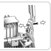
The Junction Box is provided for each FFHP Luminaire. The Junction Box will be mounted to the back of the FFHP Luminaire. Use the wiring diagram provided to properly wire the luminaire to the power supply.
