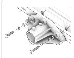
1) The ACFH280SF Slipfitter is specifically designed to withstand the weight of our FFH280. Fasten the two bolts to the trunnion of the FFH280 and properly tighten the bolts to ensure the slipfitter will not be loosed up throughout time.
