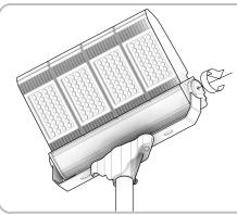
3) Once the slipfitter is properly secured into place to the pole, the electrician can now adjust the Tilt angle of the light by losing up the bolts on the side of the luminaire. and tilting the light to its desired Tilt. Once the tilt is as desired, tighten the two side bolts to lock its position in place.
