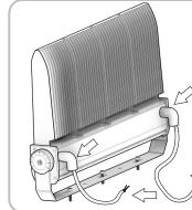
3. There should be two cables sticking out of the back of the fixture in order for it to be installed. Remove the two PVC pipe elbows from the fixture. The purpose of these elbows is to protect the cable during shipping.
