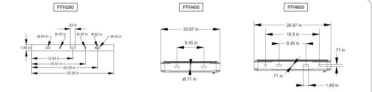
1. Depending on the model number, the FFH will determine which Trunnion Mount hole dimensions will have to be followed.
