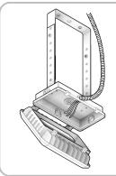
9. Run the flexible conduit through the opening on the FCPG back box and lock it into the conduit plug opening. Extend the power supply cables inside the conduit to be connected to the LED Driver inside the FCPG.
