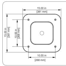
1) Drill [4] small holes 10.55" OC. using this template. At the center of the 4 holes, also cut a notch on the ceiling to allow the wiring from the FCPB to be powered with the AC Power Supply cable. Minimum notch size is 1.5" diameter hole. (As long as there is access to wire above the ceiling.
