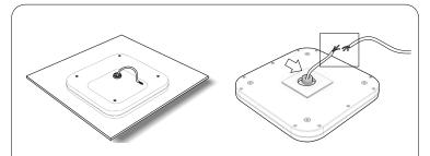
2) Feed the center cable from the FCPB through the center notch on the ceiling and connect the cables with the AC Power Supply Cable. Be sure to make all connections inside a j-box. (J-Box not included). Follow the Wiring Diagram below for more inststructions.
