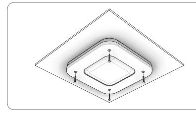
3) Once everything is properly wired, the last step is to fasten the FCPB to the ceiling .Use the [4] provided bolts to fasten the FCPB. This step must be checked by a qualified engineer to make sure the luminaire is safely secured into place.
