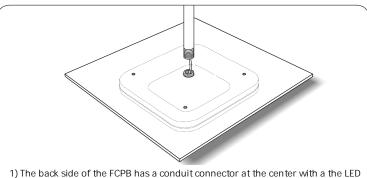
1) The back side of the FCPB has a conduit connector at the center with a the LED Driver Input cable sticking out. This luminaire can be installed by simply threading a 3/4" Conduit to the back side. This can be done once the FCPB is flush to the ceiling or without any ceiling surface present.
