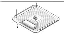
2) Fasten the two Angles provided to the FCPA luminare. Also, install the LED Driver to the FCPA. This is done by screwing one screw to secure the Driver to the light. Double sided tape can be used for more support. (Tape not Included)
