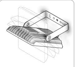
5. Adjust the tilt angle on the FALB to get the light beam pointing towards the desired location.
