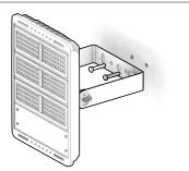
4. Fasten the AC-ALB-FM2 Flood Mount bracket to the mounting surface using the appropriate mounting bolts. (not included)
