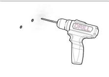
Drill holes on the mounting surface by following the Drilling Template to mount the AC-ALB-FM2 flood mount to the desired height.
