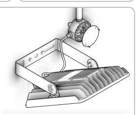
7. The FALB power cable must be fed into a Junction Box specific for outdoor applications. Follow the wiring diagram provided to install the FALB to the power cable. All wiring must be done inside the J-box and all cables must be fed through a water-proof connector. All wiring must be installed by a certified electrician and must be compliant to NEC standards.
