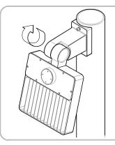
7. Adjust the Tilt Angle on the F2SB luminaire, once the Tilt Angle is as desired, finish tightening the Socket Head bolt to firmly tighten the F2SB with the Arm Mount.
