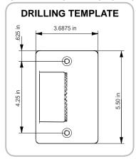
1. Use provided Hole Pattern for drilling. Make sure to make an extra notch for the power cables to run through the Round Tube.
