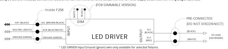
If the Ground Wire is missing and the Power Supply includes a ground wire, connect the power supply ground wire to the fixture.
