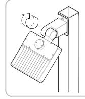
7. Adjust the Tilt Angle on the F2SB luminaire, once the Tilt Angle is as desired, finish tightening the Socket Head bolt to firmly tighten the F2SB with the Arm Mount.
