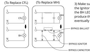
3) Make sure to take off the Ballast ( along with the Ignitor and capacitor) before installing the BH LED bulb, otherwise the ballast will produce the resonance of high voltage and eventually make the BH Light bulb fail.
