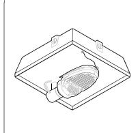
6) As an extra safety precaution, The 75W-115W BH Series comes with a small round clip attached to the front tip of the bulb. This clip can be used to install a Security cable. Clip the Security cable to the small clip and fix the other end to the fixture base frame. This method can also be used to prevent the lamp from slanting downward for its own weight.
