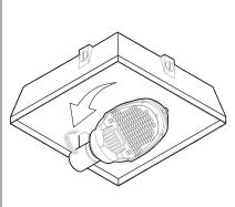
5) After the base has been properly screwed into place, if the orientation of the bulb is not facing down, its housing is able to rotate to the appropriate orientation while the lamp base stays intact.
