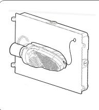
6) As an extra safety precaution, The 75W-115W BH Series comes with a small round clip attached to the front tip of the bulb. This clip can be used to install a Security cable. Clip the Security cable to the small clip and fix the other end to the fixture base frame. This method can also be used to prevent the lamp from slanting downward for its own weight.
