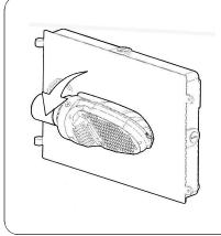
5) After the base has been properly screwed into place, if the orientation of the bulb is not facing down, its housing is able to rotate to the appropriate orientation while the lamp base stays intact.
