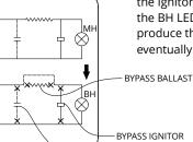
3) Make sure to take off the Ballast ( along with the Ignitor and capacitor) before installing the BH LED bulb, otherwise the ballast will produce the resonance of high voltage and eventually make the BH Light bulb fail.
