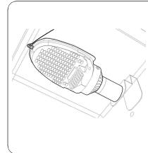
6) As an extra safety precaution, The 75W-115W BH Series comes with a small round clip attached to the front tip of the bulb. This clip can be used to install a Security cable. Clip the Security cable to the small clip and fix the other end to the fixture base frame. This method can also be used to prevent the lamp from slanting downward for its own weight.
