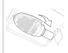
5) After the base has been properly screwed into place, if the orientation of the bulb is not facing down, its housing is able to rotate to the appropriate orientation while the lamp base stays intact.
