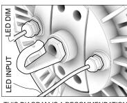
THIS DIAGRAM IS A RECOMMENDATION ON HOW TO INSTALL THE WIRING INSIDE THE JUNCTION BOX. APPLY WATERPROOF SEALANT AFTER ALL WIRING IS COMPLETE.
