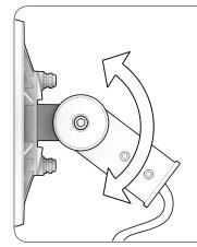
STEP 4: Before completely tightening the two parts of the slip-fitter together, make sure to orient the angle designed. Once you have adjusted the Slip-fitter to the desired orientation, fasten the M12 bolt.
