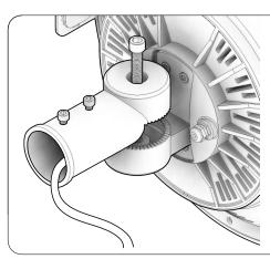
STEP 3: Using the M12 Machine Screw, Run the cables from the FHW, through the ACHWSF Slipfitter.
