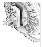
STEP 2: Fasten the ACHWSF part with the [4] mounting holes using the same socket head machine bolts that were removed in Step 1.
