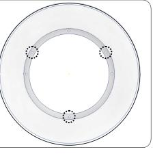
STEP 2: Using a Phillips Screw Driver, Fasten the [3] provided machine screws from the inside portion of the 90° reflector to secure it into place.
