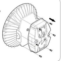
2. When the back housing is removed, the electrician will be able to see the LED Driver connected to the LED Board. This cable to be left alone. There should also be an Input Cable connected to the LED DRIVER connected with a Splicing Connector. Unclip the wires of the LED Driver from the Splicing Connector.
