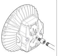
4B. Once the cable is running outside the center opening, the electrician can now screw in the ACHUCM adaptor and the cables are able to be connected to a power outlet conduit.
