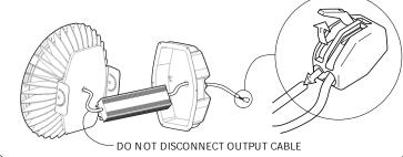
3. Using a #2 Phillips screw driver, remove the (2) M4-07 x 6 mm Low Profile Pan Head Machine screws from the LED Driver Locking Strip. This will give you access to the opening in back of the housing in order to run the cables from the LED Driver Input through the opening.
