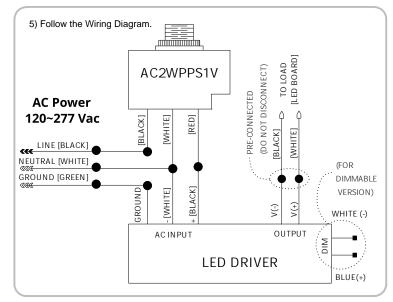
6) Use Wire Nuts, Wire Connectors, or Butt Splices at P.O.C. All Connections must be sealed for moisture. Let the Black wire from the photocell run out from the back side of the Back Box since it will be getting connected to the hot wire from the AC Power supply. Use a 3-way connector for the white wires and bring them out from the back side. Run the ground wire out if its on the LED Driver. (Wire Connectors not included)
