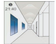
Light remains in dimming level at night.
