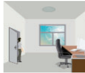
Sufficient natural light. Light does not switch on.
