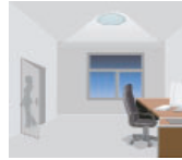
When natural light is below daylight threshold. After Hold-Time, light dims to Stand-By level.
