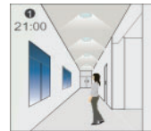
Movement detected. Light switches on at 100%.
