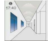
Natural Light is insufficient (no motion). Light turns on automatically at i.e. 10%.
