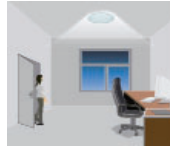
Insufficient natural light. Sensor switches light on automatically when presence detected.
