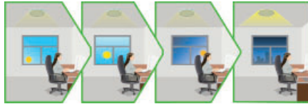
Based on the the level of natural light available, the light output is regulated. The light turns on at full or dims to maintain the lux level.
