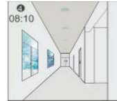
Natural light level exceeds setpoint off. Light will turn off even when space is occupied.
