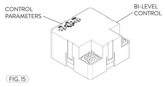
The Mounting Bracket is pre-installed and secured to the inside of the FSWA fixture. The Bi-Level Occupancy Control fits directly on the Mounting Bracket (Fig. 16).
