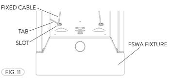
Once the tabs have been inserted, the FSWA fixture will be safely secured in place for mounting (Fig. 12).
