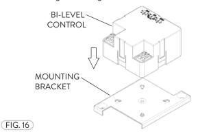
3 The Control Parameters are adjustable on the Sensor or by a wireless Commissioning Device. The Control Parameters allow the user to adjust the Mode (A thru E), Dimming (10% thru 100%), and Time (30 sec thru 30 min) Level (Fig. 17). The Control Modes are given in more detail in the next column.
