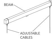
Using the Aircraft Cable (with tabs on both ends), insert the tabs into the FSWA fixture Slots on both sides (Fig. 11) .
