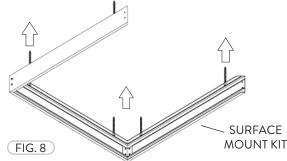
Slide in the FPNB Fixture through the open side of the Surface Mount Kit. This is when all the wiring installations should be made as well. Please refer to the wiring diagram on the front page for wire installation instructions.
