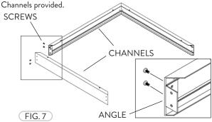
(2) Fasten the three Channels to the ceiling surface. Bolts not provided.
