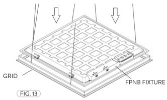
Carefully mount the FPNB Fixture to the recessed Grid and adjust any Aircraft Cables if necessary.
