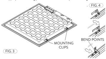
Insert the luminaire onto the T-Bar ceiling grid. Secure safety cable to connection holes as needed to meet local seismic requirements. Safety cable and method of attachment to the building provided by contractor according to local building codes.
