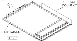
Once the FPNB Fixture is properly installed on the Surface Mount Kit, fasten the last two angles and side Channel with Screws to completely enclose the FPNB Fixture.
