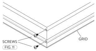
Notch out the ceiling drywall surface. Insert the preassembled
