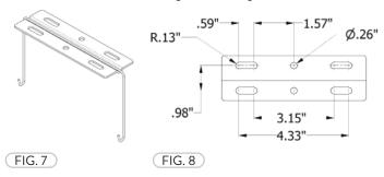
Install the Surface Hanger Mounts (2) to a Level Mounting Surface/Ceiling with the Mounting Bolts (not included) (Fig. 9). Once the Surface Hanger Mounts are installed onto the Level Surface/Ceiling and properly secured, place Hooks through the holes on each side of the FLHQ fixture (Fig. 10).
