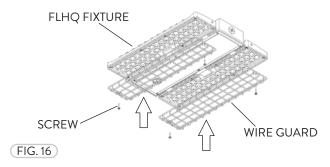
Use the Screws to fasten the Wire Guard into the holes located at each end of the fixture lens (Fig. 17).
