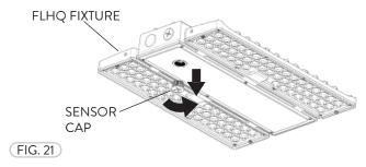
The Lighting Control Sensor has a 'Plug and Play' Connector that inserts into the bottom of the FLHQ fixture (Fig. 22).
