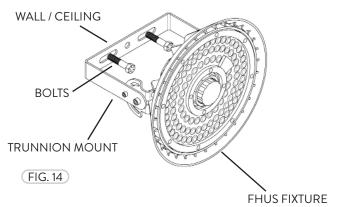
Instead of having the fixture directly surface mounted to a fixed position, the FHUS fixture can be adjusted by loosening the screws at the sides of the of the Trunnion Mount. Rotate the FHUS Fixture to the desired tilt angle to aim at a specific position. Tighten the screws to firmly tighten the FHUS Fixture to the Trunnion Mount (Mounting Bolts not included).
