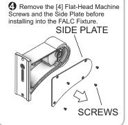
Run the FALC Cable through the inside the Arm Mount. Align the hole and teeth from the Arm Mount with the FALC Bracket Mount and use the Socket Head Screw to fasten them together at the appropriate Fixture tilt angle.
